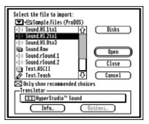
The displayed list of files is built by calling each translator's TrFilter routine (TrFilter uses the data in the GetDirEntry record to form a rating value on its ability to translate the file). The checkbox determines what range of files is displayed.
