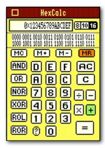
The HexCalc calculator has a traditional layout, with the keypad in the centre, function keys surrounding it, and a Display showing the result of the calculation at the top. It also has a simple Memory Save and Recall function.
